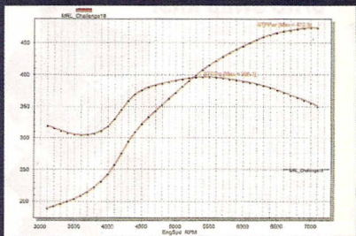
The 340 Mopar was a popular choice this year, and engine builder Mike Liston of MRL Performance brought a powerful one to the 2010 contest. With a flat-tappet camshaft, this little powerhouse made more than 470 horsepower.
