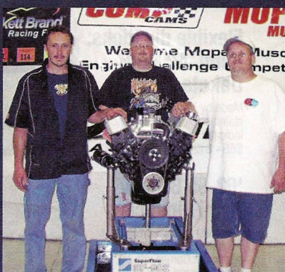
As a newcomer to the AMSOIL/Mopar Muscle Engine Challenge, B&G Speed and Machine built a flat-tappet 360 for the contest. At more than 418 horsepower, their small-block Mopar made 1.14 horsepower per cubic inch.
